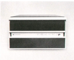
9867A Single-Platter or 9867B Dual-Platter Mass Memory (Disc Drive)
